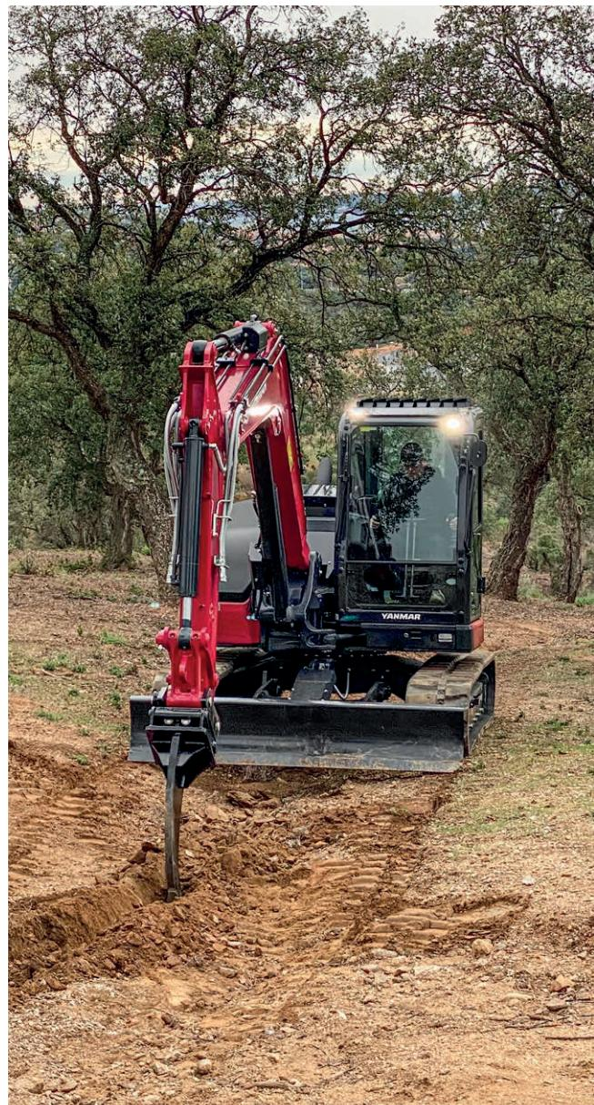
\*Test performed with buckets of 600mm width, on the same soil (gravel), site and weather conditions, with 3 different operators on each excavator digging a trench 0,8m depth during 10min.
