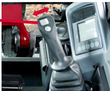
2 Proportional PTO control lever
