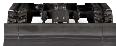
Extended undercarriage: 1280 mm
