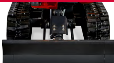
Extended undercarriage: 1 000 mm
