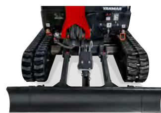
Extended undercarriage: 1 380 mm
