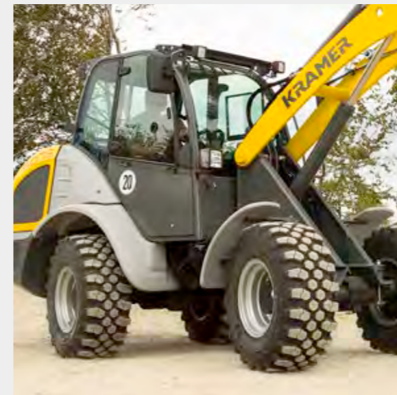
Crab steering for precise positioning
